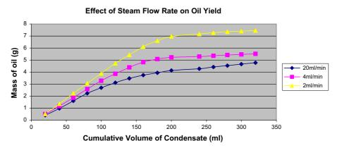
Fig. 8. Lavender oil cumulative yield curves at different steam flow rates.
