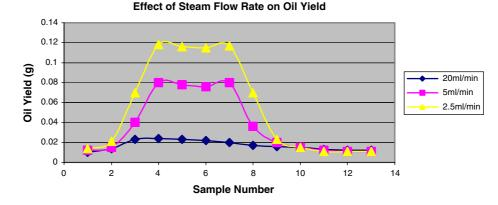
Fig. 5. Artemisia oil sample yield curves at different steam flow rates.
