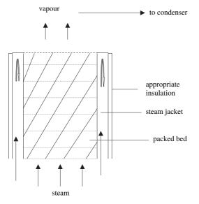
Fig. 1. Diagram of the new packed bed extraction system developed and tested to improve extraction efficiency and product quality.
