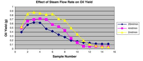
Fig. 7. Lavender oil sample yield curves at different steam flow rates.
