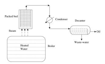
Fig. 2. Diagram of the steam distillation extraction process.
