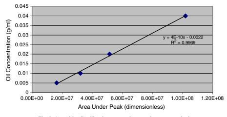
Fig. 3. Artemisia oil calibration curve using camphor-L as standard.
