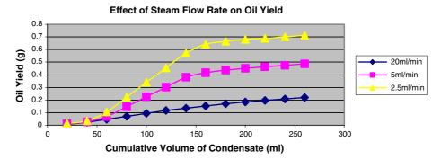
Fig. 6. Artemisia oil cumulative yield curves at different steam flow rates.
