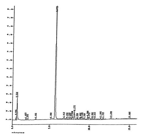
Fig. 9. Chromatogram of water-soluble components in artemisia oil.
